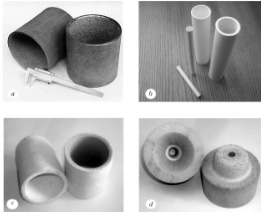
Fig. 7. Articles produced by the pulse method of pressing with account for the curves of the dynamic compressibility of powder materials: a) porous titanium filters; b) ceramic filtering elements and porous diaphragms for reactors of chemical treatment of water in an "Izumrud" plant; c) refractory one- and two-layer crucibles for melting and pouring ferrous and non-ferrous metals; d) two-layer batch-beakers made from ZrO_2 and Al_2O_3 for continuous casting machines.
